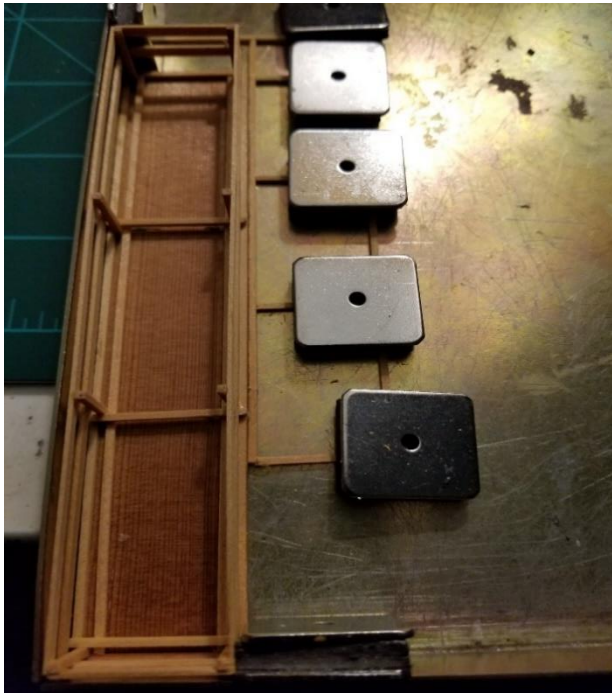
A magnetic gluing jig is used to square the floor of the boxcar and loading dock and holding the parts in place and flat while drying. The jig is from Micro Mark, part #60304
